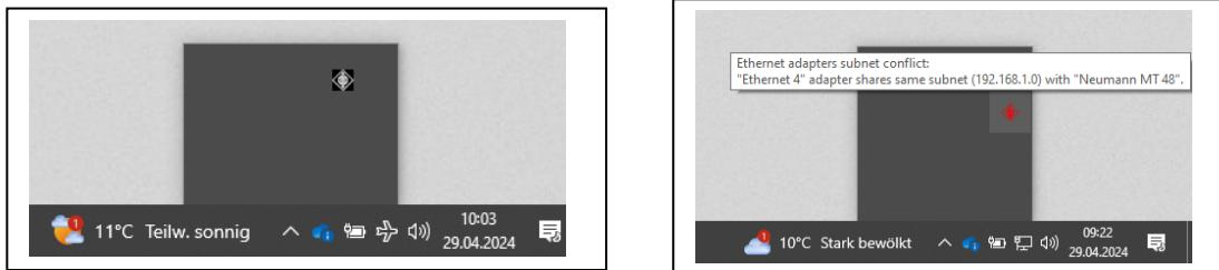
**To avoid this conflict, the USB and RJ45 connection of the MT48 should not be used simultaneously if there is already another connection established to the router via another primary network card or WLAN.**
